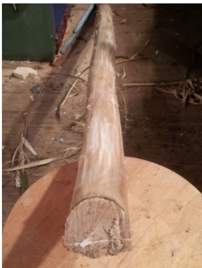
Wych Elm stave: Note the small diameter, giving a very rounded back
